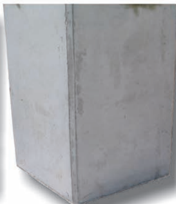
With Oztec Rebar Shaker® in congested rebar
