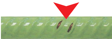
Damage caused by a standard steel vibrator head.
