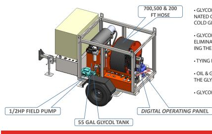
• GLYCOL GETS UP TO OPERATING TEMPERATURE FASTER THAN COMPETITORS (DESIG-NATED CIRCULATION PUMP PULLS FROM THE RESERVOIR AND DOESN'T HAVE TO PUSH COLD GLYCOL THROUGH THE FIELD HOSES)
