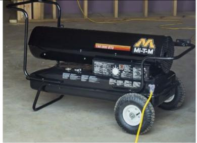
**MOTOR** Heavy-duty, cast aluminum enclosed electric motor
