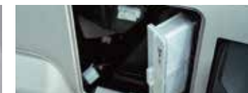
Air conditioner filter can be easily removed without tools for cleaning. One for outside air and one for inside air.
