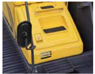
Front mounted three steps instead of only two for easy safe access.
