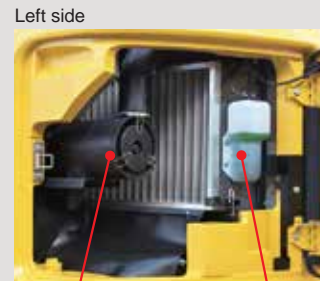
Left side Radiator reservoir tank Air cleaner ● Easy access to cooling units
