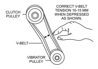
Figure 10. V-Belt Tension
