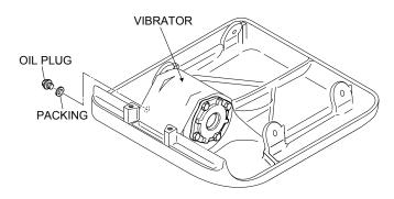
Figure 11. Vibrator Oil Check
