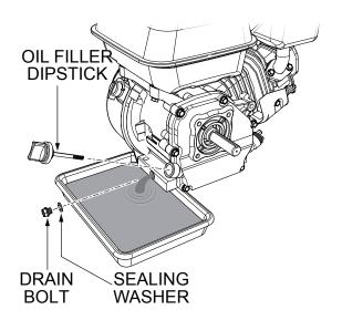
Figure 28. Draining Engine Oil
