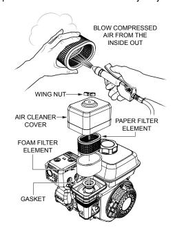
Figure 24. Engine Air Filter (Dual)
