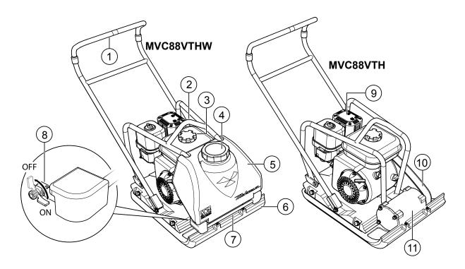
**Figure 2. Plate Compactor Components**
