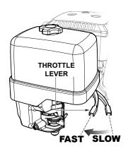
Figure 13. Throttle Lever (1/3 Start Position)
