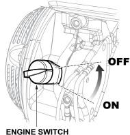
Figure 22. Engine ON/OFF Switch (OFF Position)
