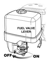
Figure 23. Fuel Valve Lever (OFF)
