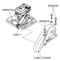
Figure 8. V-Belt Cover Removal
