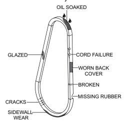
Figure 9. Drive Belt Inspection
