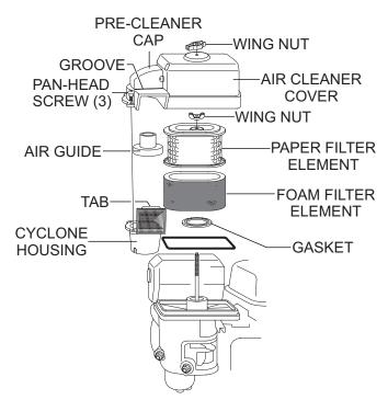
Figure 25. Engine Air Filter (Cyclone Type1)
