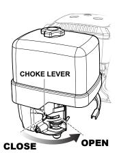
Figure 14. Engine Choke Lever (Open)
