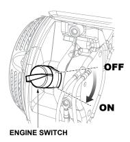
Figure 16. Engine ON/OFF Switch (ON Position)
