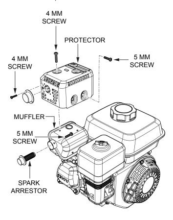
Figure 31. Spark Arrester Removal
