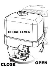
Figure 15. Choke Lever (Closed)
