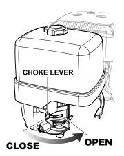
Figure 18. Choke Lever (Open)
