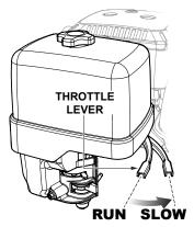
Figure 21. Throttle Lever (Slow/Idle Position)
