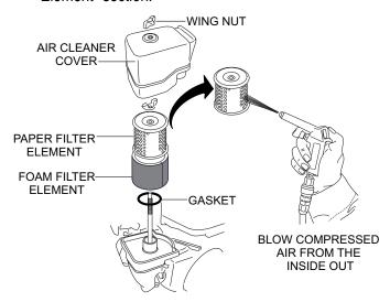
Figure 26. Engine Air Filter (Cyclone Type 2)
