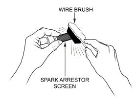
Figure 32. Cleaning The Spark Arrester
